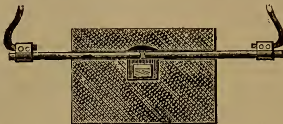
FIG. 50.—MOISSAN'S ELECTRIC FURNACE (CROSS-SECTION).
